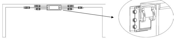
Step 2. Connect the input 1 port of the RSD-D to the PV module junction box, and connect the input 2 port of RSD-D to the other PV module junction box.
