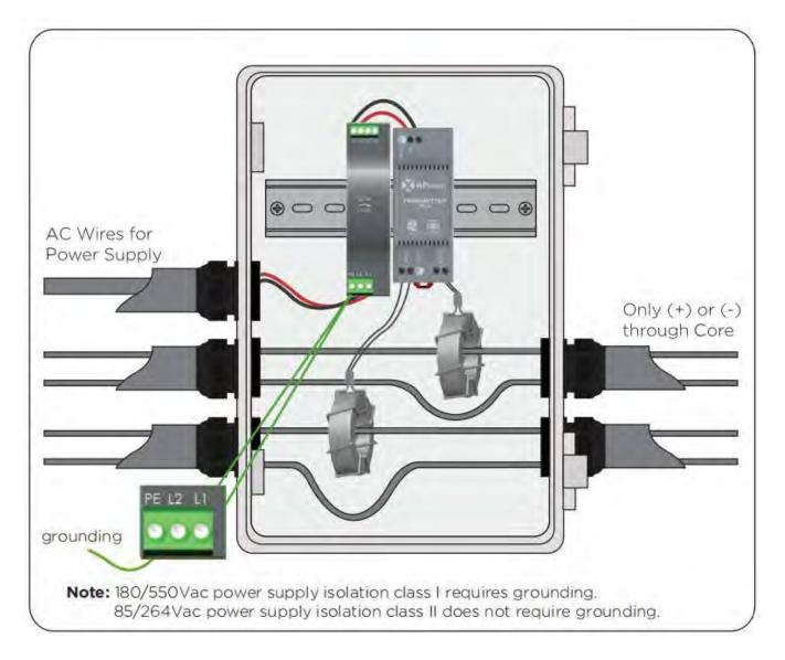
Note: Install the RSD-D before powering on the Transmitter-PLC.
