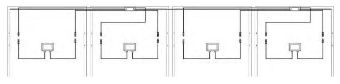
WARNING: When connecting the RSD-D to only one PV module, use INPUT1 port ONLY, then connect a DC extension cable to both terminals of INPUT2 to short the unused side, otherwise the RSD-D may be damaged.
