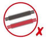
Do not put all the PV+ or all the PV- together in the same cable tray VS
