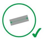
If multiple rapid shutdown systems use the same cable tray, the length of the cable tray should be kept as short as possible (less than 3m)
