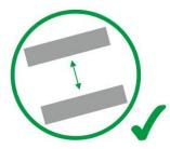
The cable trays for two different rapid shutdown systems should be installed as far apart as possible ( more than 20cm )
