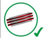
The PV +& PV - of the same string should be placed as twisted-pair in a cable tray
