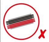
Do not separate PV + and PV - in a cable tray
