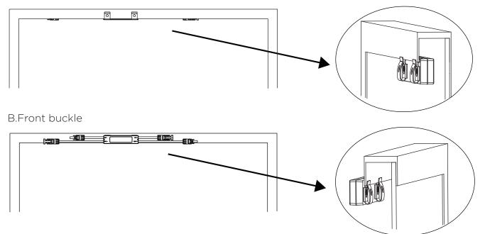
NOTE: Do not place the RSD-S-PLC (including DC connectors) where exposed to the sun, rain or snow, even gap between modules. Allow a minimum of 3/4"(1.5cm.) between the roof and the bottom of the RSD-S-PLC to allow proper air flow.
