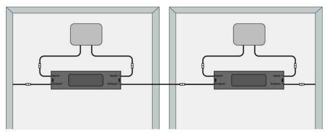
NOTE: Do not short-circuit the RSD-S-PLC output connectors, otherwise it will be damaged. NOTE: When installing RSD-D cable, the bending radius of the cable near the casing must be greater than 50 mm.
