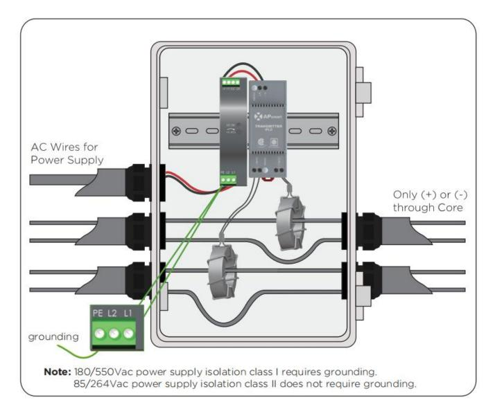
Note: Install the RSD-S-PLC before powering the Transmitter-PLC. Note: The waterproof jacket and related accessories are not configured before delivery and customers need to buy by themselves.
