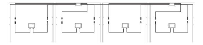
*NOTE: When installing RSD-D cable, the bending radius of the cable near the casing must be greater than 50 mm.*
