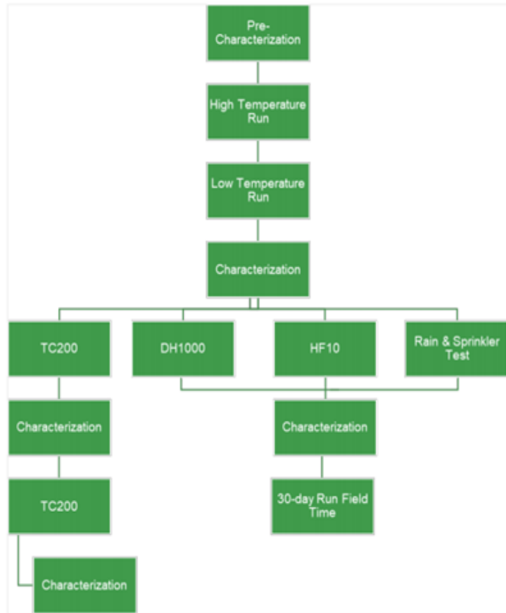
Figure 2-1: Test plan process diagram
