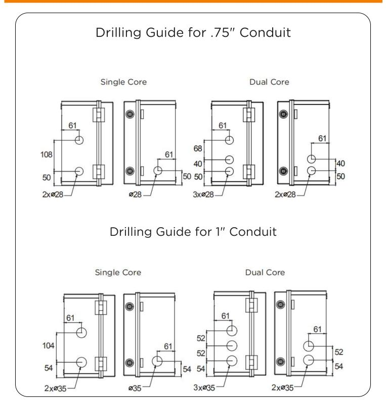
Note: The Outdoor Kit was not punched before delivery and customer need to make it themselves according to the actual situation. The figure is only for reference.
