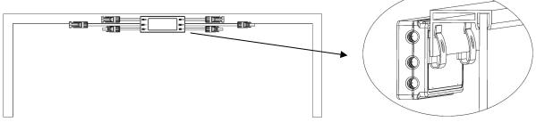
NOTE: Do not place the RSD-D (including DC connectors) where exposed to the sun, rain or snow, even gap between modules. Allow a minimum of 3/4"(1.5cm.) between the roof and the bottom of the RSD-D to allow proper air flow.
