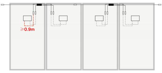
NOTE: When installing RSD-D cable, the bending radius of the cable near the casing must be greater than 50 mm.
