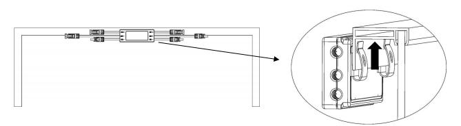
NOTE: Do not place the RSD-D (including DC connectors) where exposed to the sun, rain or snow, even gap between modules. Allow a minimum of 3/4"(1.5cm.) between the roof and the bottom of the RSD-D to allow proper air flow.
