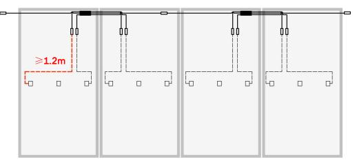
NOTE: The output cable length of integrated junction box PV module should be no less than 0.9m.
