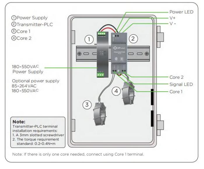
Transmitter-PLC power supply must be on same AC branch circuit as inverter to meet rapid shutdown requirements.
