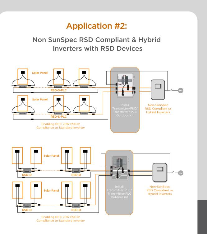
In Non SunSpec RSD Compliant & Hybrid Inverters system, a Transmitter device (Transmitter-PLC / Transmitter-PLC Outdoor Kit) needs to be installed together with RSD Devices (RSD-S-PLC & RSD-D) to realize module-level rapid shutdown function.
