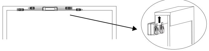
NOTE: Do not place the RSD-S-PLC (including DC connectors) where exposed to the sun, rain or snow, even gap between modules. Allow a minimum of 3/4"(1.5cm.) between the roof and the bottom of the RSD-S-PLC to allow proper air flow.
