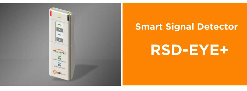
The RSD-EYE+ is a small and lightweight multifunctional handheld detection device for sensing pulse modulation from the power line communication (PLC) signal between transmitter and RSD, to ensure compliance to the SunSpec Alliance Rapid Shutdown protocol. In addition, the RSD-EYE+ can also be used as a handheld transmit device, by connecting an optional external DC cable to send an in-line keep-alive signal to the RSD.
