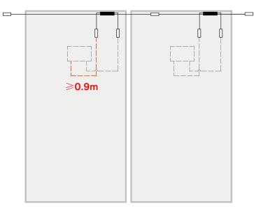
NOTE: When installing RSD-S cable, the bending radius of the cable near the casing must be greater than 50 mm.
