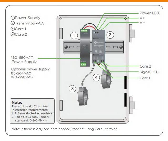
Transmitter-PLC power supply must be on same AC branch circuit as inverter to meet rapid shutdown requirements.
