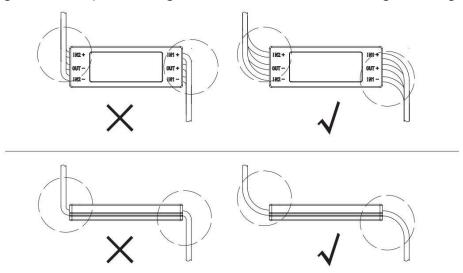
Step 3: Connect the output ports of two adjacent RSD-Ds in series and then connect to the inverter with a self-made DC extension cable.
