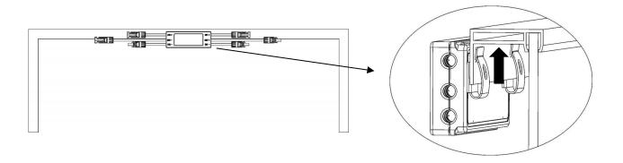
NOTE: Do not place the RSD-D (including DC connectors) where exposed to the sun, rain or snow, even gap between modules. Allow a minimum of 3/4"(1.5cm.) between the roof and the bottom of the RSD-D to allow proper air flow.
