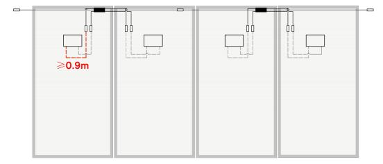
NOTE: When installing RSD-D cable, the bending radius of the cable near the casing must be greater than 50 mm.
