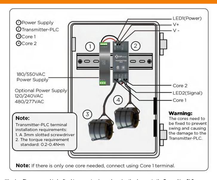
Warning: The cores need to be fixed to prevent swing and causing the damage to the Transmitter-PLC.
