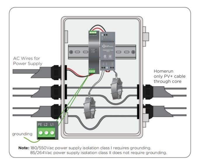
Note: Install the RSD-S-PLC before powering the Transmitter-PLC. Note: The waterproof jacket and related accessories are not configured before delivery and customers need to buy by themselves.
