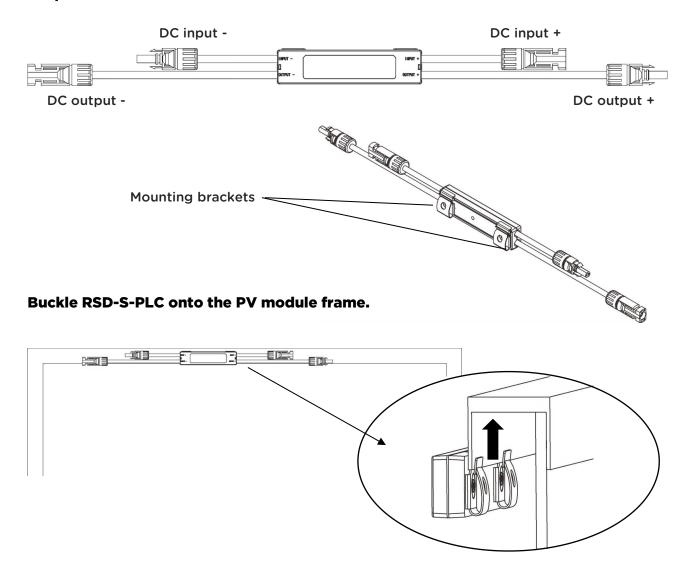
NOTE: Do not place the RSD-S-PLC (including DC connectors) where exposed to the sun, rain or snow, even gap between modules. Allow a minimum of 3/4"(1.5cm.) between the roof and the bottom of the RSD-S-PLC to allow proper air flow.
