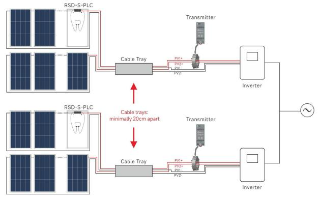
Do not place wires from different inverters in the same cable tray. Asynchronous signals may cause crosstalk and lead to abnormal system behavior.
