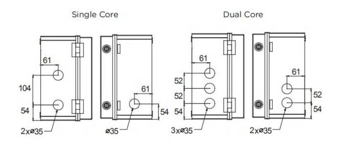
NOTE: The Outdoor Kit was not punched before delivery and customer need to make it themselves according to the actual situation. The figure is only for reference.
