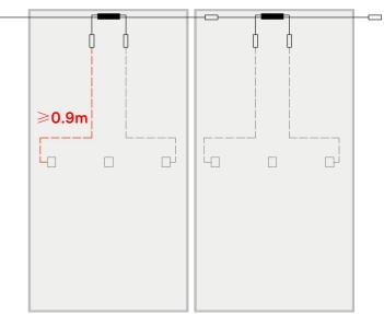
NOTE: The output cable length of integrated junction box PV module should be no less than 0.9m.
