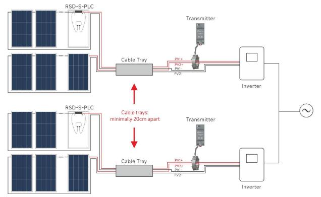
Do not place wires from different inverters in the same cable tray. Asynchronous signals may cause crosstalk and lead to abnormal system behavior.
