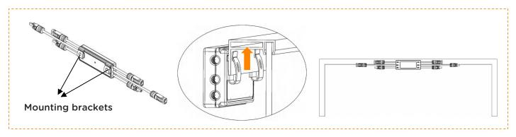
**NOTE:** Do not place the RSD-D (including DC connectors) where exposed to the sun, rain or snow, even gap between modules. Any surface of the RSD other than the mounting bracket must be at least 15mm away from surrounding objects. In particular, it is forbidden to have DC cables run close to or cover the RSD-S-PLC casing.
