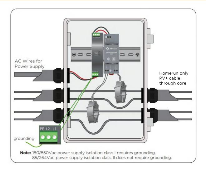
**NOTE:** Install the RSD-D before powering the Transmitter-PLC.
