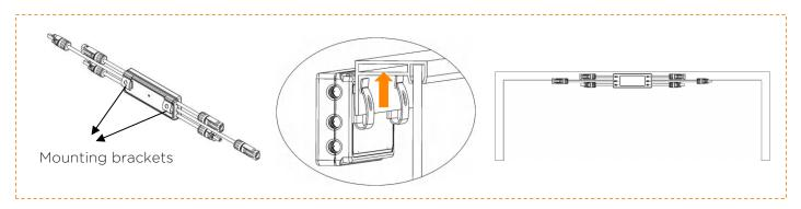
**NOTE:** Do not place the RSD-D (including DC connectors) where exposed to the sun, rain or snow, even gap between modules. Any surface of the RSD other than the mounting bracket must be at least 15mm away from surrounding objects. In particular, it is forbidden to have DC cables run close to or cover the RSD-S-PLC casing.
