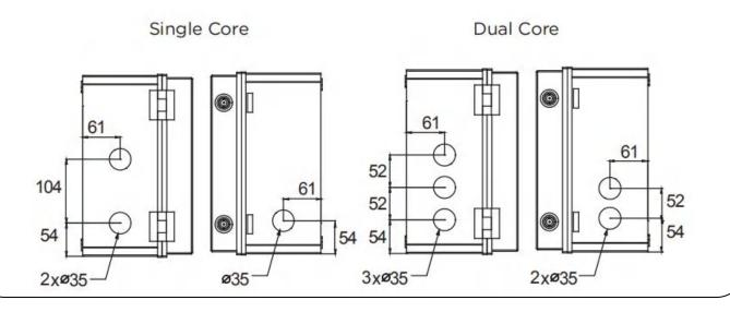
**NOTE:** The Outdoor Kit was not punched before delivery and customer need to make it themselves according to the actual situation. The figure is only for reference.
