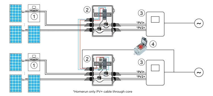
① RSD ② Transmitter-PLC-PLUS-Outdoor Kit ③ Inverter ④ Emergency stop button box(optional)\*
