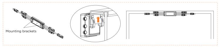
**NOTE:** Do not place the RSD-D (including DC connectors) where exposed to the sun, rain or snow, even gap between modules. Any surface of the RSD other than the mounting bracket must be at least 15mm away from surrounding objects. In particular, it is forbidden to have DC cables run close to or cover the RSD-S-PLC casing.
