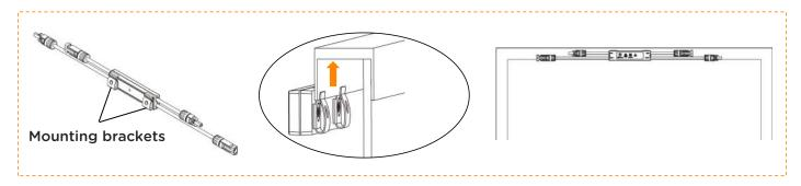
**NOTE:** Do not place the RSD-S-PLC (including DC connectors) where exposed to the sun, rain or snow, even gap between modules. Any surface of the RSD other than the mounting bracket must be at least 15mm away from surrounding objects. In particular, it is forbidden to have DC cables run close to or cover the RSD-S-PLC casing.
