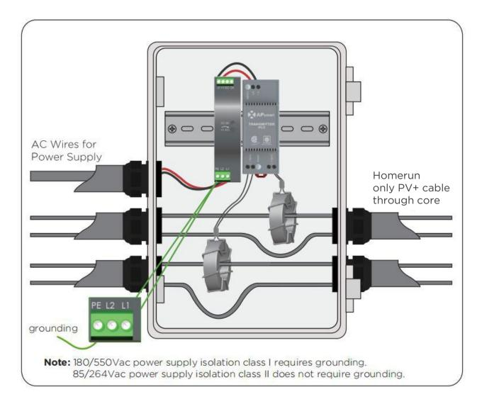
NOTE: Install the RSD-S-PLC before powering the Transmitter-PLC.
