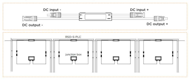
**NOTE:** Do not short-circuit the RSD-S-PLC output connectors, otherwise it will be damaged.
