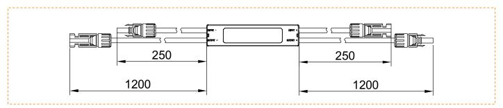
NOTE: The output cable length of triad junction box PV module should be no less than 0.9m.
