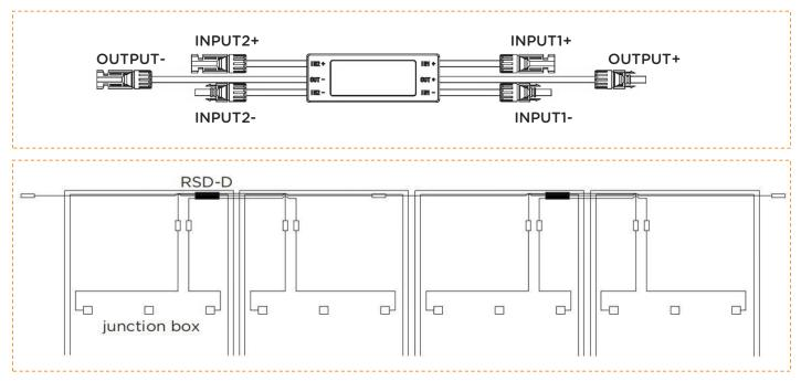
(1) RSD-D can be installed together with RSD-S-PLC;
