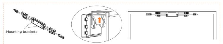
**NOTE:** Do not place the RSD-D (including DC connectors) where exposed to the sun, rain or snow, even gap between modules. Any surface of the RSD other than the mounting bracket must be at least 15mm away from surrounding objects. In particular, it is forbidden to have DC cables run close to or cover the RSD casing.
