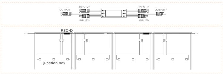
(1) RSD-D can be installed together with RSD-S-PLC;
