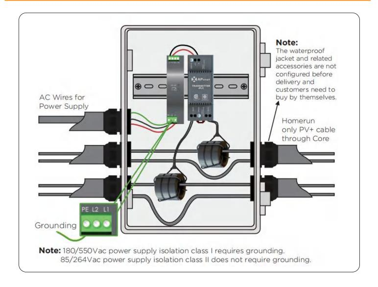
**NOTE:** Install the RSD-D before powering the Transmitter-PLC.
