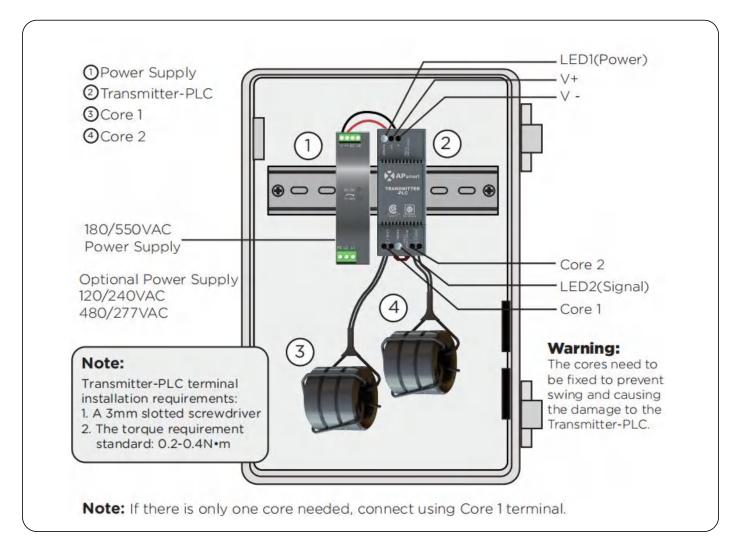
Warning: The cores need to be fixed to prevent swing and causing the damage to the Transmitter-PLC.
