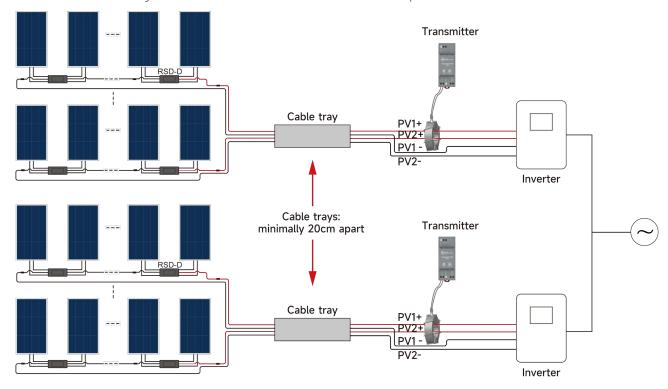
Do not place wires from different inverters in the same cable tray. Asynchronous signals may cause crosstalk and lead to abnormal system behavior.
