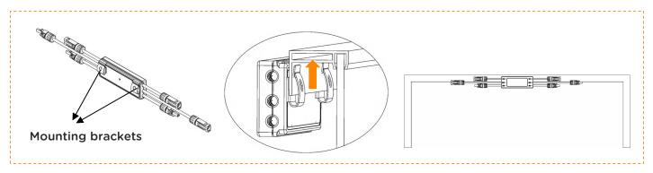
**NOTE:** Do not place the RSD (including DC connectors) where exposed to the sun, rain or snow, even gap between modules. Any surface of the RSD other than the mounting bracket must be at least 15mm away from surrounding objects. In particular, it is forbidden to have DC cables run close to or cover the RSD casing.
