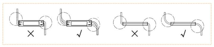
Step 3: Connect the output connectors of the RSD-S-PLC in series to the string, the string open-air DC voltage is within the range of (0.6-1V) x RSD-S-PLCs. (This range may vary due to different on-site environment.)
