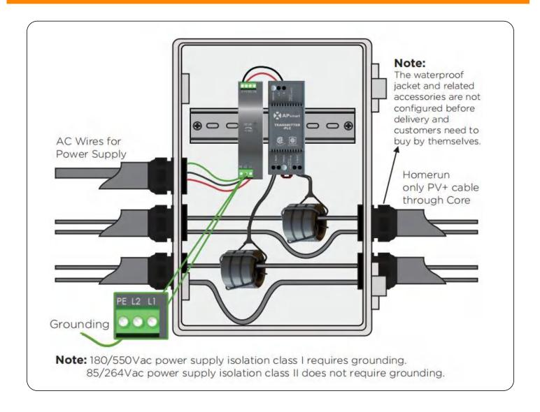
**NOTE:** Install the RSD-D before powering the Transmitter-PLC.
