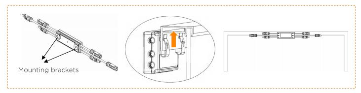
**NOTE:** Do not place the RSD (including DC connectors) where exposed to the sun, rain or snow, even gap between modules. Any surface of the RSD other than the mounting bracket must be at least 15mm away from surrounding objects. In particular, it is forbidden to have DC cables run close to or cover the RSD casing.
