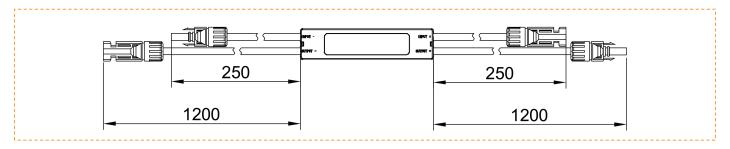
NOTE: The output cable length of triad junction box PV module should be no less than 0.9m.
