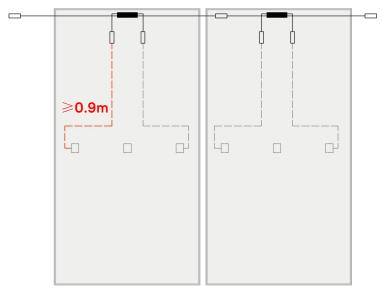
NOTE: The output cable length of integrated junction box PV module should be no less than 0.9m.
